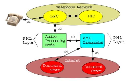
Figure 4: High-level view of the PML architecture.
