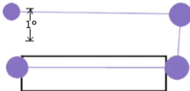
Figure 1. The participant looked at the four corners of the rectangle, but the eye tracking data are all above the corners due to systematic errors. Circles represent fixations.
