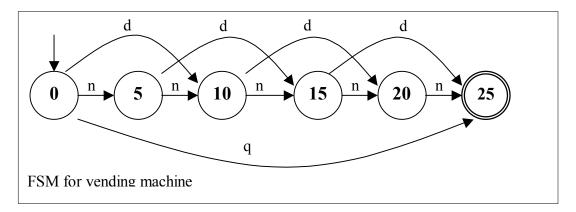
We have omitted the arrows for coin combinations that total more than 25 cents, but they could be added for each state, with all of them terminating in the accept state. Also, we could add arrows for inputs other than nickels, dimes, and quarters (call them all slugs). The arrows for such input in each state would loop back to the same state.
