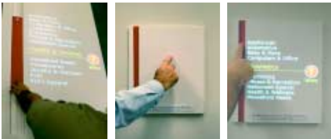
Figure 5. The Ubiquitous Product Finder. (a) projected on to a table with a physical slider; (b) user “calls” the application; (c) the paper tag becomes an interactive product finder.
