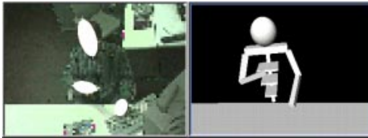
Fig. 2. Left: video and 2-D blobs from one camera in the stereo pair. Right: corresponding configurations of the dynamic model.
