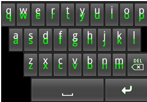
Figure 7. The two different positions of the keys' labels. The green labels show the default Android keyboard and the white labels show the elevated labels.
