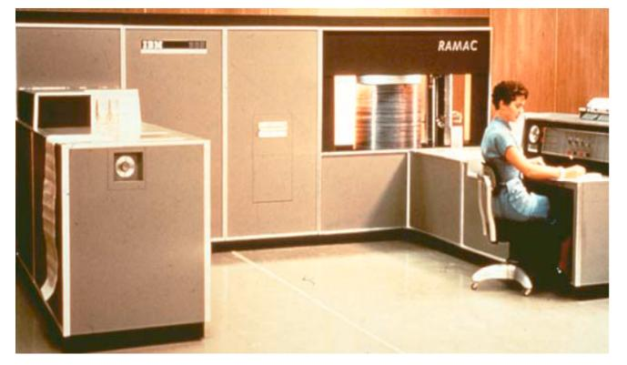
1956: IBM 305 RAMAC -5 MB capacity (50 disks, each 24" in diameter)
