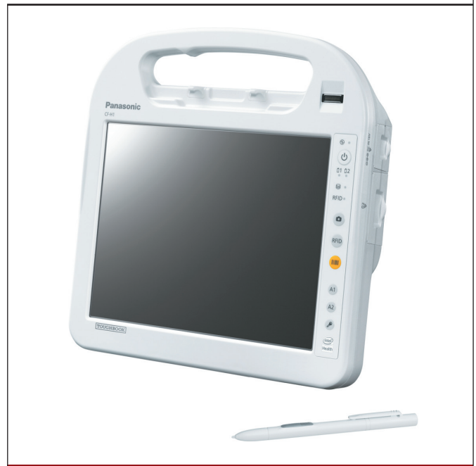
Figure 1. Designed to meet the specific needs of healthcare professionals, Panasonic’s Toughbook H1 rugged mobile clinical assistant (MCA) is the first Continua Certified application hosting device supporting Bluetooth. It features a 10.4-inch, dual-touch, 500-nit display that accepts input from a stylus or finger touch. Hot swappable twin batteries provide limitless hours of use.
