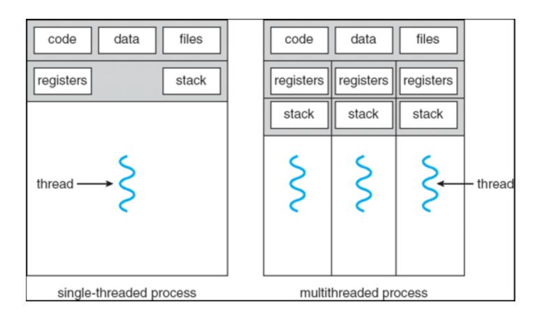
Regular UNIX process can be thought of as a special case of a multithreaded process: a process that contains just one thread
