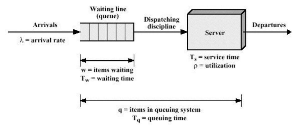
Figure A.2 Queuing System Structure and Parameters for Single-Server Queue
