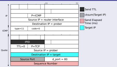
ICMP TTL exceeded replies permit recovery of: target probed, originating TTL (hop), and responding router interface at that hop.
