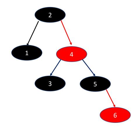
after insertion of 1,2,3,4,5,6 into empty RB tree
