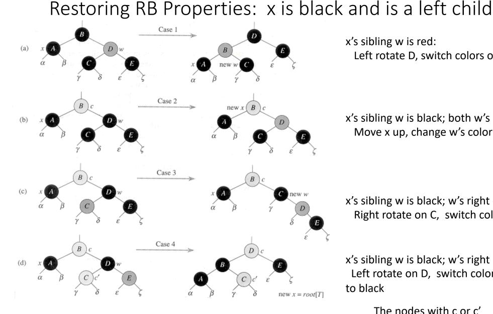
x's sibling w is red: Left rotate D, switch colors of B and D
