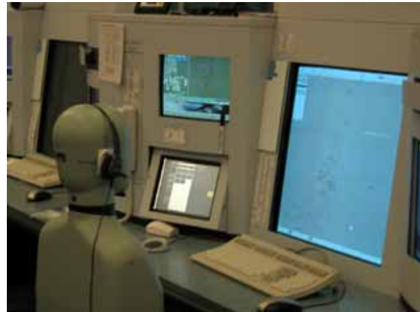
Figure 1 A TAAATS air traffic control console, with a manikin in the controller’s position.
