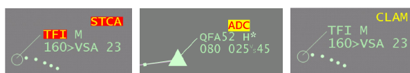
Figure 2. Examples of on-screen visual alerts (P1, P2 and P3 from left to right). The color scheme for P4 is the same as for P3.
