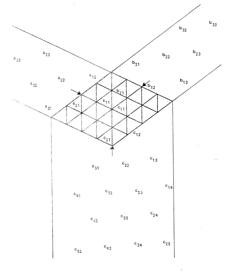
Figure 7. Triangular Processor Array for Matrix Mulitplication
