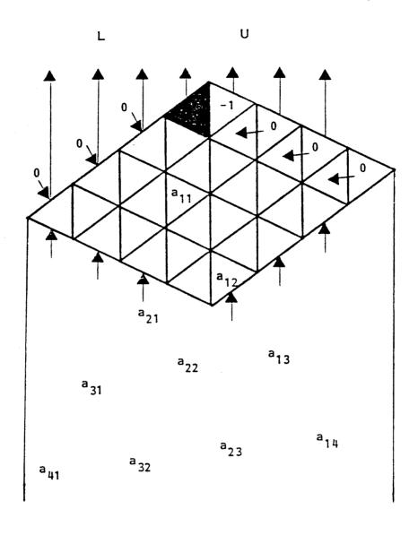
Figure 10. Triangular Processor Array for LU Decomposition
