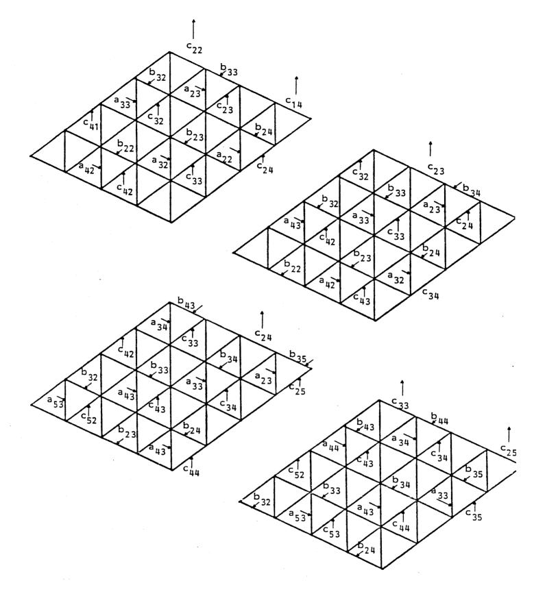
Figure 8. Four Steps in Matrix Multiplication on the Triangular Processor Array
