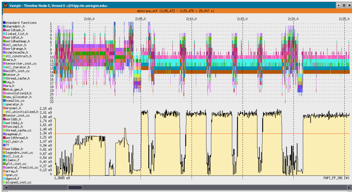
Fig. 5. MADNESS Trace for one thread shown in Vampir. Routines are colored by filename and floating point counter rates are shown at the bottom.
