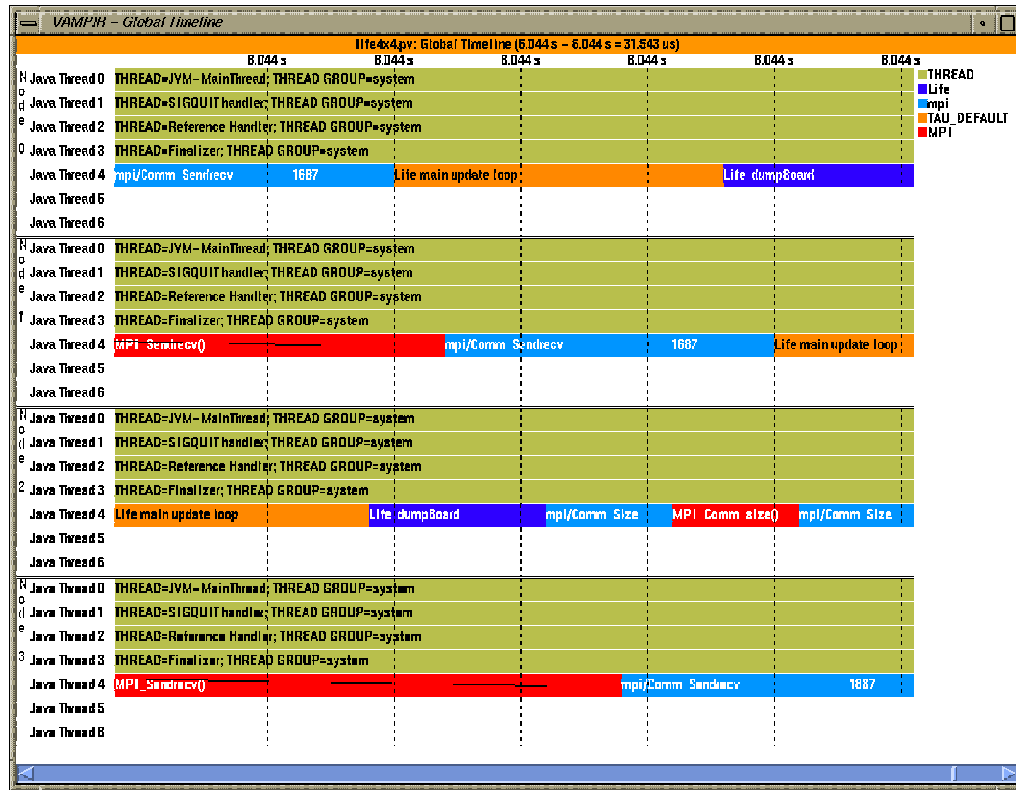
Figure 10. Performance data from source, library and virtual machine levels of a Java application
