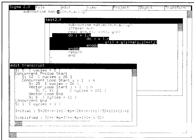
Figure 3. The Sigma restructuring tool. The programmer has highlighted the Do j loop for object-code analysis. The Edit Transcript window shows the object-code summary.
