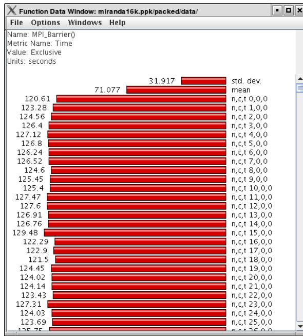
This display graphs the values that the particular function had for each thread along with the mean and standard deviation across the threads. You may also change the units and metric displayed from the *Options* menu.
