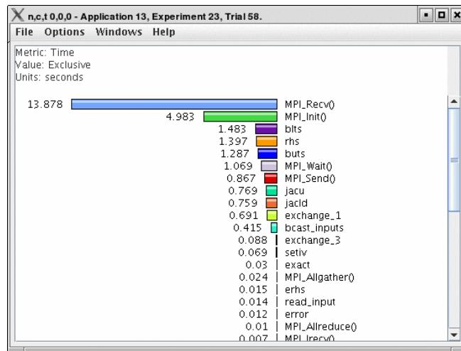
This display graphs each function on a particular thread for comparison. The metric, units, and sort order can be changed from the *Options* menu.
