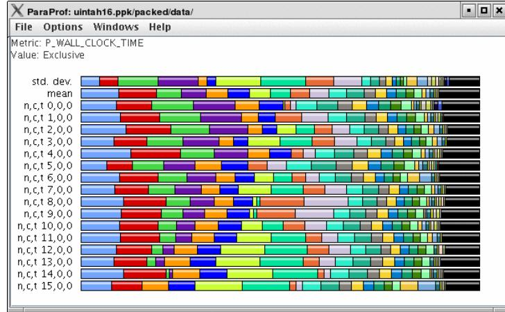
This window shows each thread as well as statistics as a combined bar graph. Each function is represented by a different color (though possibly cycled). From anywhere in ParaProf, you can right-click on objects representing threads or functions to launch displays associated with those objects. For example, in Figure 9.4, “Main Data Window”, right click on the text  $n,c,t, 8,0,0$  to launch thread based displays for node 8.
