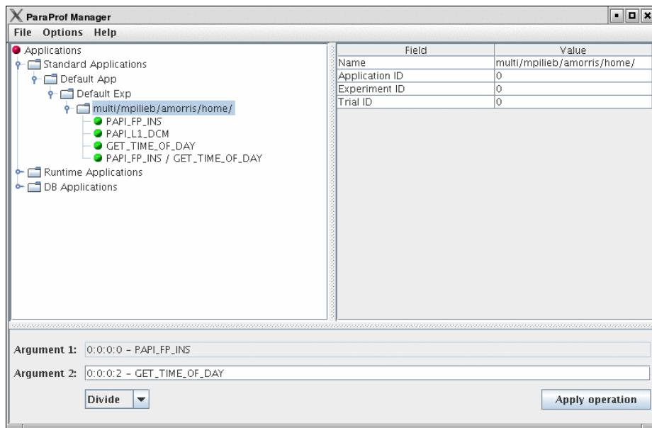
In Figure 9.3, "Creating Derived Metrics", we have just divided Floating Point Instructions by Wall-clock time, creating FLOPS (Floating Point Operations per Second). The 2nd argument is a user-editable text-box and can be filled in with scalar values by using the keyword 'val' (e.g. "val 1.5").
