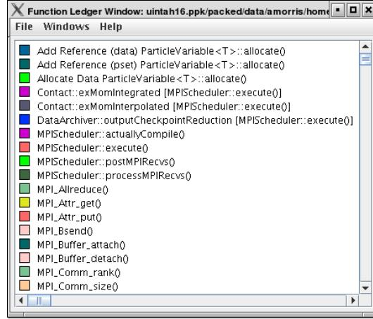
The function ledger shows each function along with its current color. As with other displays showing functions, you may right-click on a function to launch other function-specific displays.
