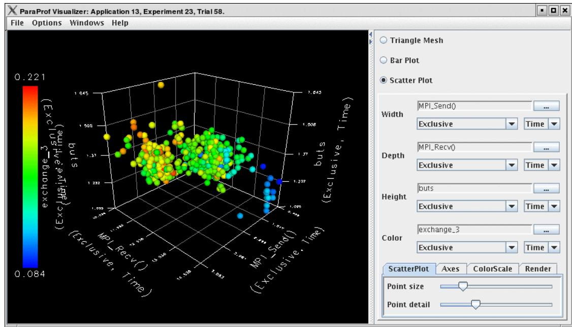
This visualization method plots the value of each thread along up to 4 axes. Each axis represents a different function and metric. This view allows you to discern clustering of values and relationships between functions across threads.
