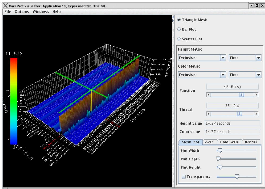
This visualization method shows two metrics for all functions, all threads. The height represents one chosen metric, and the color, another. These are selected from the drop-down boxes on the right.
