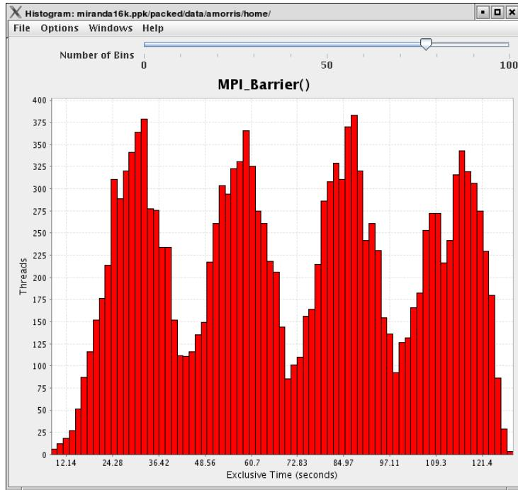
This display shows a histogram of each thread's value for the given function. Hover the mouse over a given bar to see the range minimum and maximum and how many threads fell into that range. You may also change the units and metric displayed from the *Options* menu.
