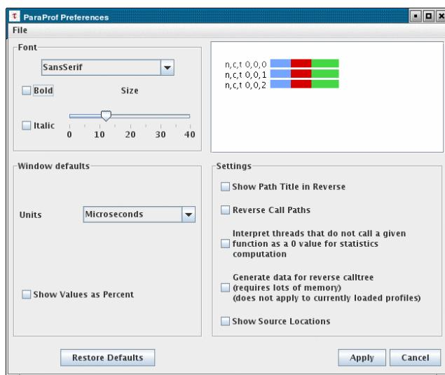
The preferences window allows the user to modify the behavior and display style of ParaProf's windows. The font size affects bar height, a sample display is shown in the upper-right.
