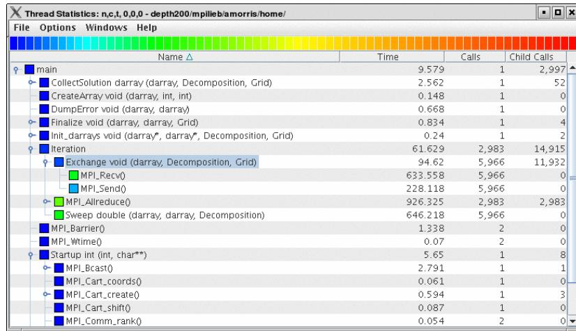
The display can be used in one of two ways, in "inclusive/exclusive" mode, both the inclusive and exclusive values are shown for each path, see Figure 11.3, "Thread Statistics Table, inclusive and exclusive" for an example.
