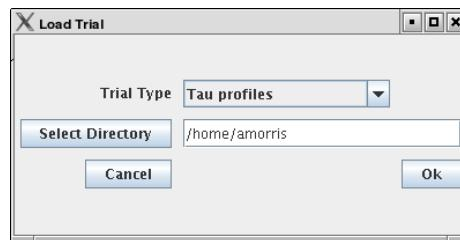
Select the type of data from the "Trial Type" drop-down box. For TAU Profiles, select a directory, for other types, files.
