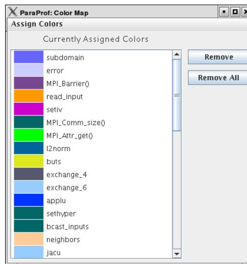
The color map shows specifically assigned colors. These values are used across all trials loaded so that the user can identify a particular function across multiple trials. In order to map an entire trial's function set, Select "Assign Defaults from ->" and select a loaded trial.
