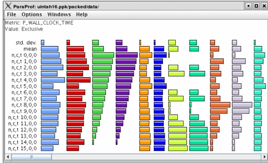
You may also turn off the stacking of bars so that individual functions can be compared across threads in a global display.
