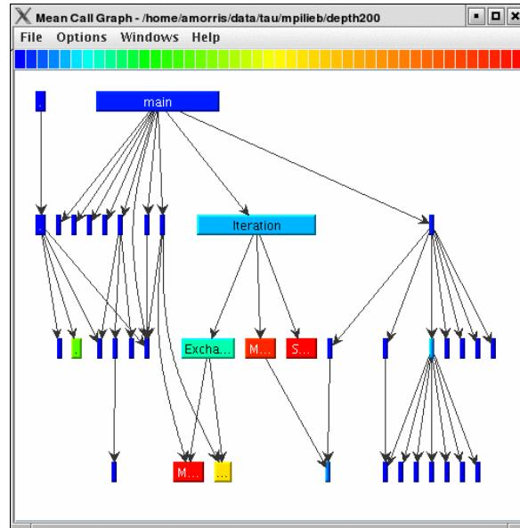
This display shows callpath data in a graph using two metrics, one determines the width, the other the color. The full name of the function as well as the two values (color and width) are displayed in a tooltip when hovering over a box. By clicking on a box, the actual ancestors and descendants for that function and their paths (arrows) will be highlighted with blue. This allows you to see which functions are called by which other functions since the interplay of multiple paths may obscure it.
