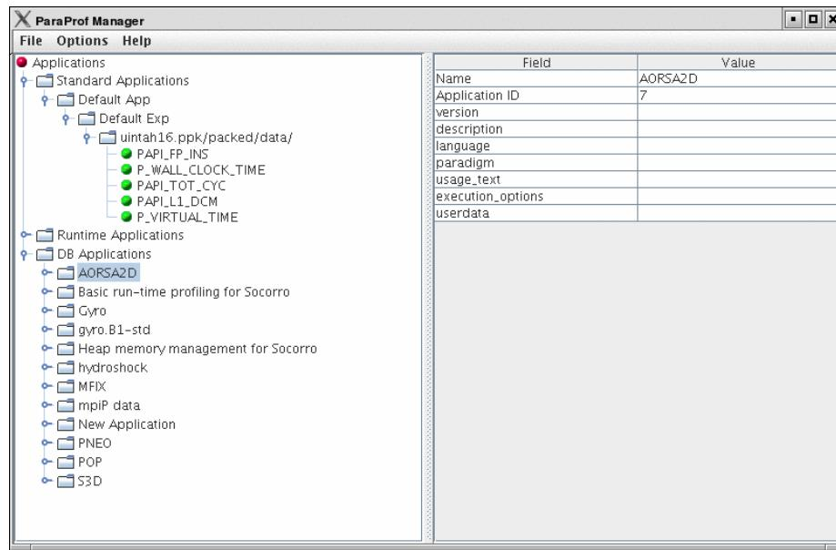
This window is used to manage profile data. The user can upload/download profile data, edit meta-data, launch visual displays, export data, derive new metrics, etc.
