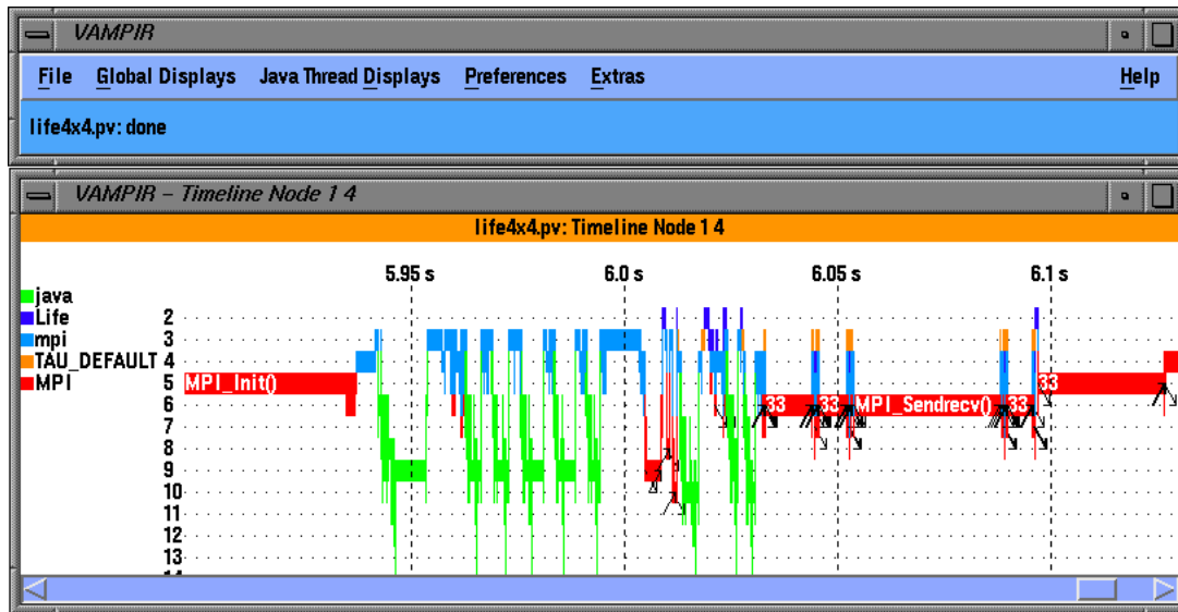
Figure 7. Vampir timeline display can show the depth of routine nesting of the callstack on a particular thread
