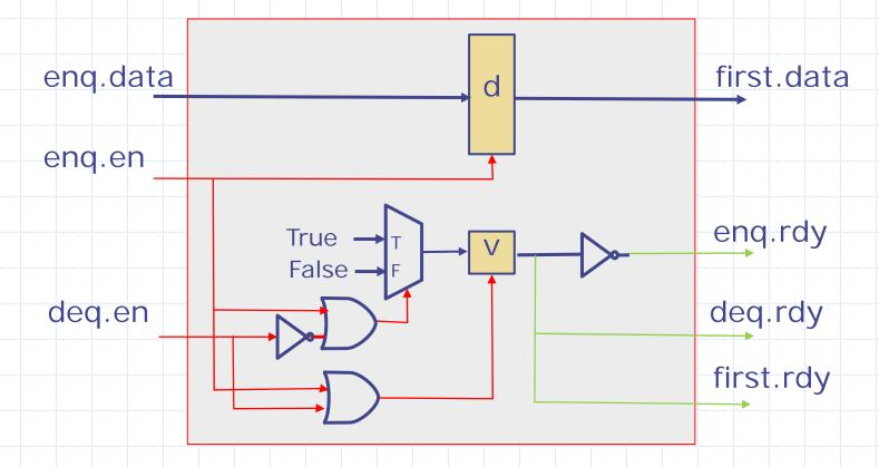
A module is a sequential circuit with input and output wires corresponding to its interface methods
