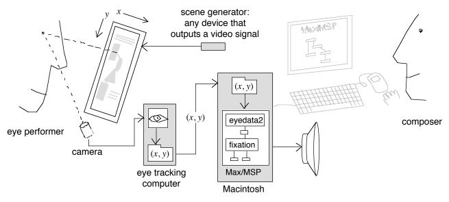
Figure 1. The EyeMusic system architecture is designed to get the human eye movement data to the musician in a context and format that are most useful for composing and performing. Arrows indicate the flow of data.
