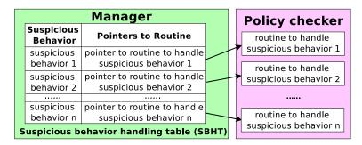
Fig. 3: Diagram of the suspicious behavior handling table (SBHT)
