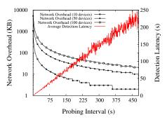
Fig. 8: The effect of probing interval on network overhead and detection latency for SVELTE
