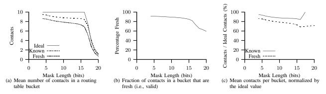
Fig. 3. Properties of routing table buckets in Kad, as a function of how specific the bucket's mask is
