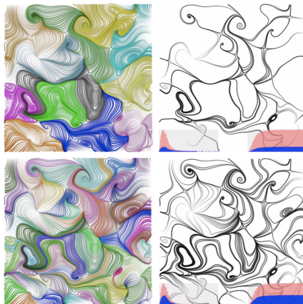
Fig. 19: Results of the hierarchical bundling visualization algorithm [68]. Left: hierarchical clustering of the flow field using 12 (top) and 70 (bottom) clusters. Right: A representative set of streamlines. Boundary streamlines of clusters are used and they highlight saddles in the flow.
