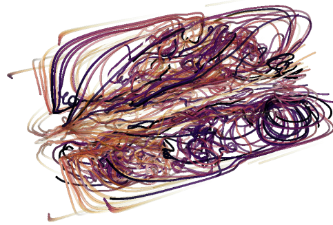
Figure 3: Streamlines rendered over a slice of the jet plume data. The jet plume is a simulation of a jet of high-velocity fluid moving into a medium at rest, created using the Gerris Flow Solver [Pop03].
