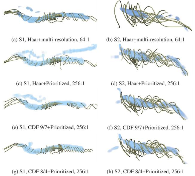
Figure 10: Renderings of local dynamics of two structures: S1 (left) and S2 (right). Visual inspection shows that the Haar+multi-resolution wavelet setting (a) and (b) at compression ratio 64:1 yields comparable results as other wavelet settings using prioritized coefficients at compression ratio 256:1.
