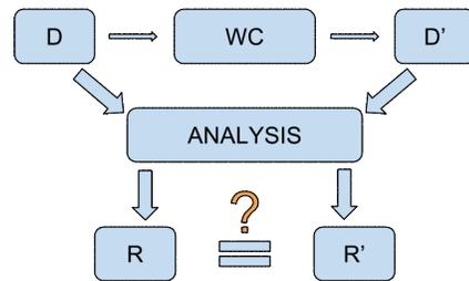
Figure 2: Our experiment methodology.  $D$  denotes the raw data,  $WC$  denotes an operator that applies wavelet compression to the data (with VAPOR),  $D'$  denotes the newly created wavelet data,  $ANALYSIS$  represents the analysis performed (with VisIt or VAPOR), and  $R$  and  $R'$  represent the results of the analysis for  $D$  and  $D'$  respectively. Our study then evaluated the difference between  $R$  and  $R'$ .
