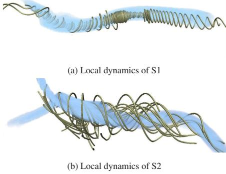
Figure 9: Visualizations of local dynamics. Streamlines are seeded in the velocity field in areas of high vorticity, showing the distinct local dynamics of the two structures. On the top (and referred to as S1), streamlines twist tightly around the core; these types of structures were identified by low mean helicity. On the bottom (and referred to as S2), streamlines writhe around the core; these types of structures were identified by high mean helicity.
