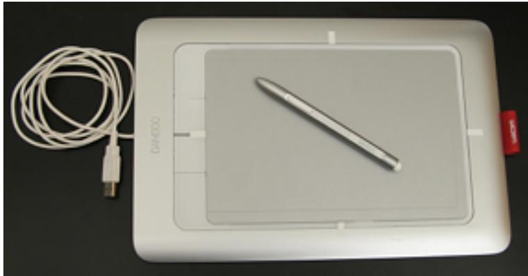
FIGURE 5.4. A Wacom Bamboo tablet and stylus served as the input device in this experiment. Tactilely distinct markers were placed at the midpoint of each side of the tablet as reference points.
