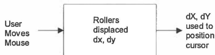
Figure 13. Block diagram of a mouse indicating how the mouse's movement turns rollers.
