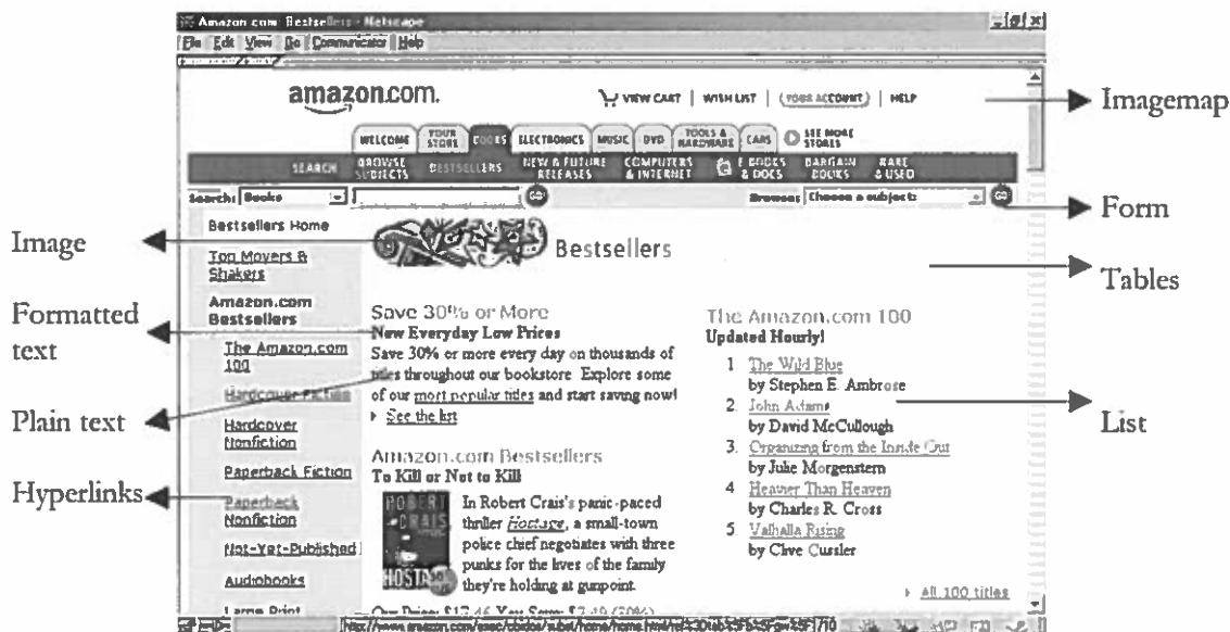
Figure 3. Element Types Found on a Typical (Amazon.com) Web Page 2,3 .
