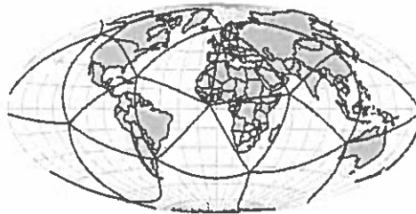
Figure 6b. Spherical icosahedron oriented using Fuller's Dymaxion orientation. Note that all vertices fall in the ocean.
