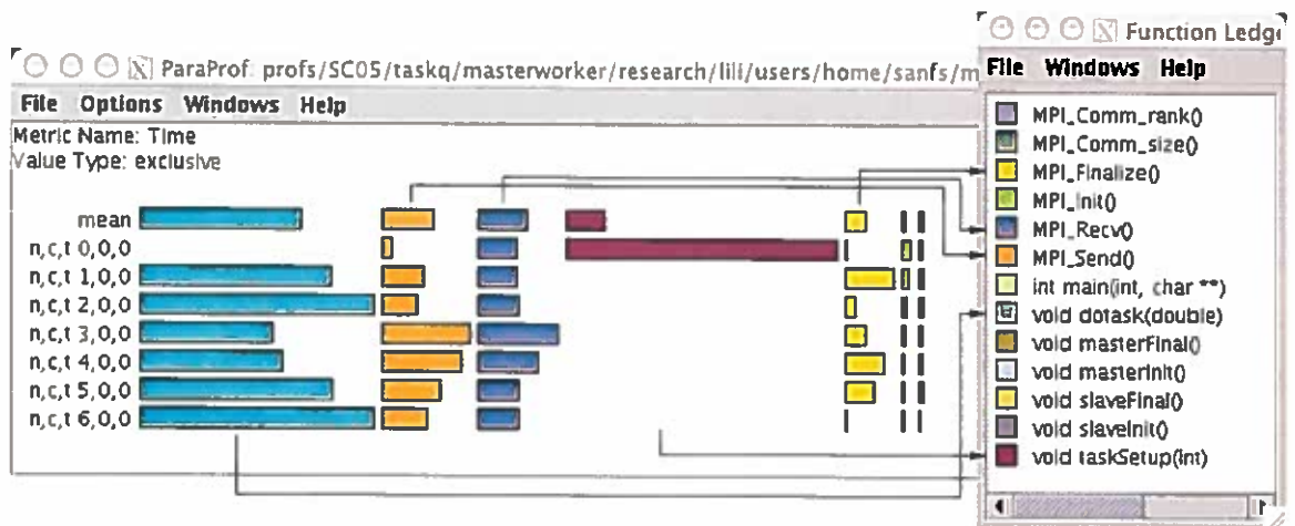
FIGURE 5.8: Paraprof graphical display of relative time spent in each function on each node, context, thread in the M-W experiment.
