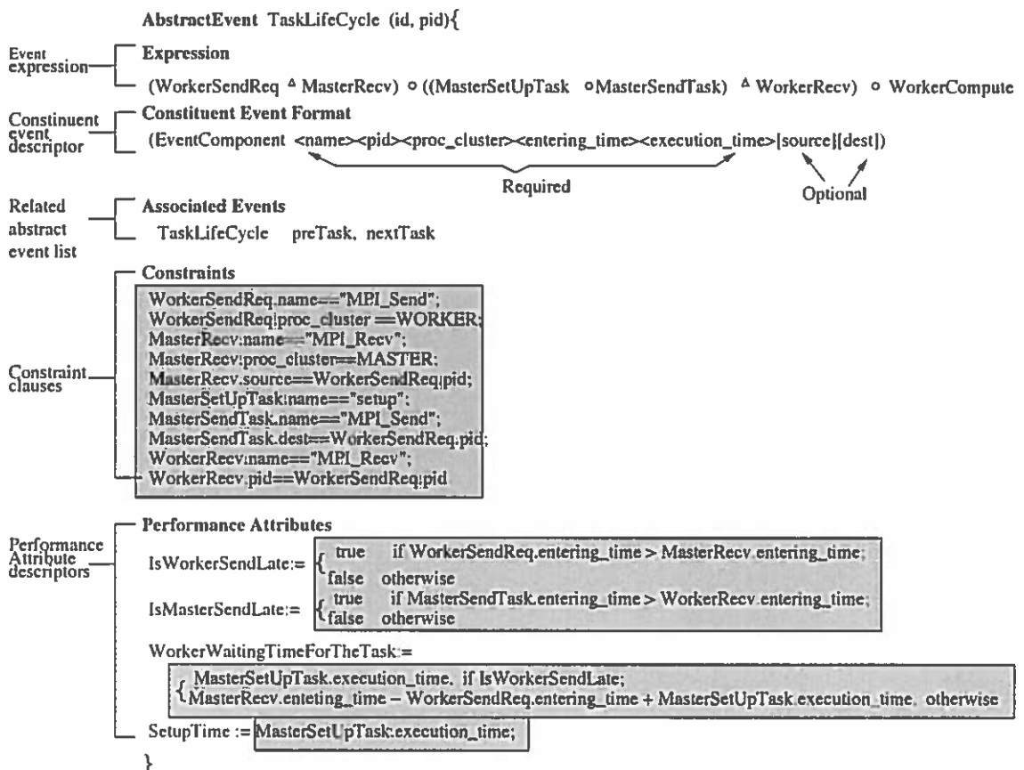
FIGURE 5.4: An abstract event description of Master-Worker model. The shaded areas are instantiated by a model implementation.
