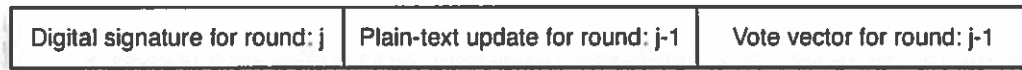
FIGURE 3.2: NEO update with voting: The format of a NEO update includes the digital signature of the update for round j , the update for round j-1 , and the vote vector for round j-1 . Note that the update includes information such as the round number so that NEO can easily determine which update belongs to which round.
