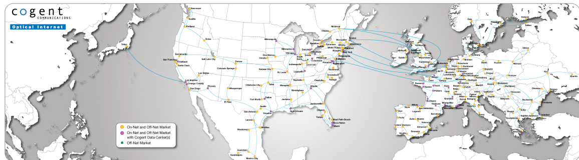
FIGURE 6.54. The PoP-level topology of Cogent retrieved from http://www.cogentco.com/files/images/network/network_map/networkmap_global_large.png in September 2013
