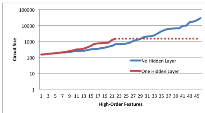
FIGURE 5.3. The number of edges in the circuit versus the number of high-order features for GACs with multilayer perceptron with no hidden layer and one hidden layer.
