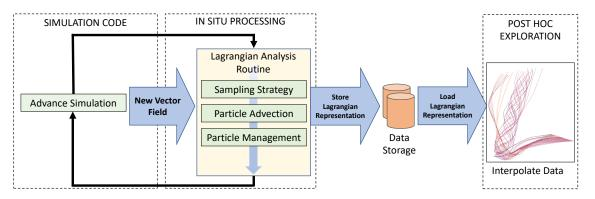
Figure 32. Schematic diagram of the **L-ISR-PHE** workflow showing in situ processing, data storage, and post hoc exploration.
