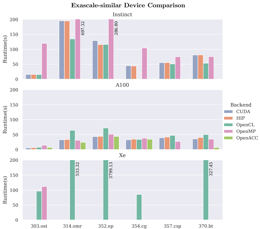
Figure 31. Absolute runtime performance comparison of different programming models (generated from OpenACC source code via OpenARC) on each device. Missing bars indicate an unsupported programming model or a failed compilation/execution.
