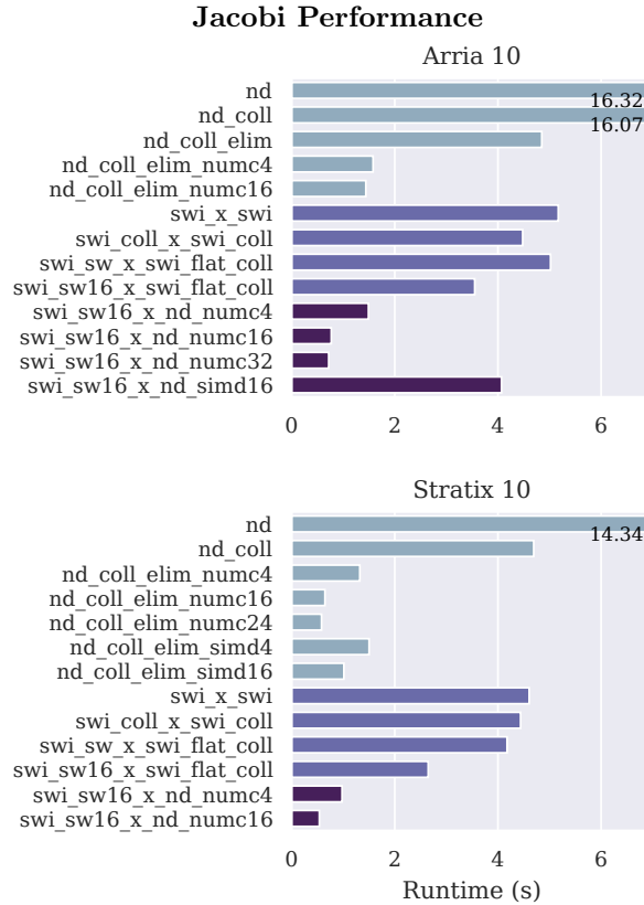
Figure 16. Runtime performance (in seconds) of Jacobi with different FPGA-specific optimizations applied (Arria 10 and Stratix 10). Blue bars indicate the multi-threaded approach, purple bars indicate the single work-item approach, and green bars indicate a hybrid multi-threaded+single work-item approach (smaller is better).
