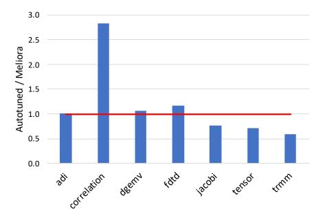
*Figure 26.* Comparison with empirically tuned performance. Values greater than one indicate that Meliora-based optimizations outperformed the empirical autotuner.
