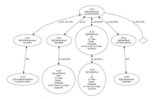
*Figure 10.* Loop structure from a C++ source code AST fragment (ROSE-generated graph).
