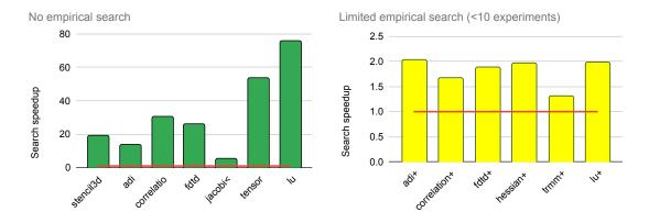
Figure 31. Comparison with empirically tuned performance. Left: Melioraguided optimizations applied without empirical search (technically the speedup is infinity, but here we show the overall time of evaluating the code version). Right: Restricted empirical autotuning, limiting the search around the Meliora-identified parameters.
