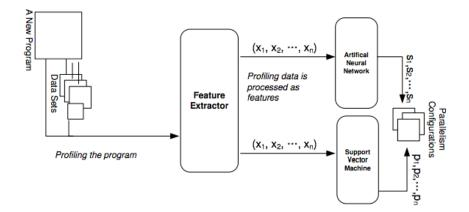
Figure 5. The workflow for parallelism mapping. From [137]
