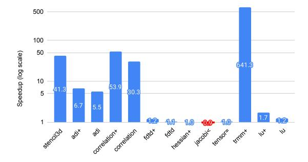
Figure 29. Speedup of Meliora-matched optimizations w.r.t. a baseline version using default parameters and compiler optimizations. In all cases except for jacobi, the Meliora versions were at least as fast as the base version, which uses the default optimization parameters in Table 10.
