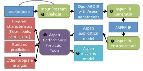
Figure 3. Workflow of the COMPASS framework. From [79]
