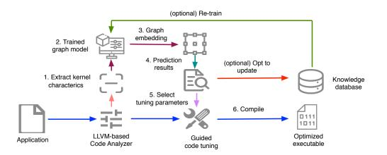
*Figure 21.* Meliora's workflow for code representation-based model generation and optimization.
