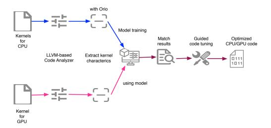
Figure 28. Unified workflow for CPU/GPU code optimization.
