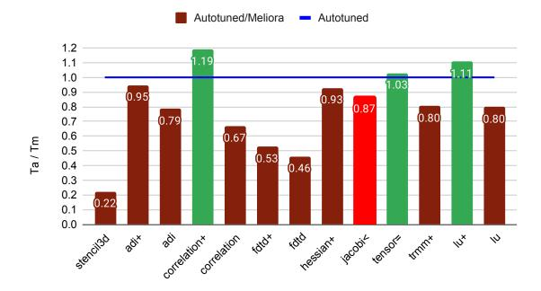
Figure 30. Ratio of autotuning execution time (Ta) to Meliora-based execution time (Tm) of the SPAPT benchmarks. The green bars (values above 1.0) indicate that Meliora-based versions outperformed the traditionally autotuned versions. Values smaller than 1.0 indicate that autotuning can yield additional benefits. In all cases except for jacobi, the Meliora versions were faster than the base version.
