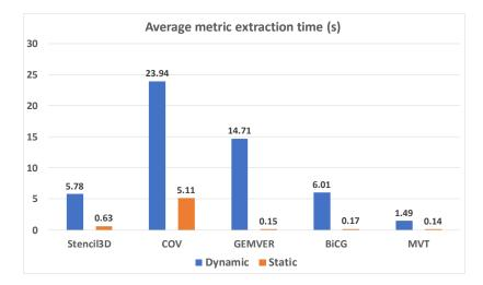
*Figure 27.* Comparison between the static and dynamic strategies for metric extraction. The X-axis lists the kernels and the Y-axis is the time in seconds.
