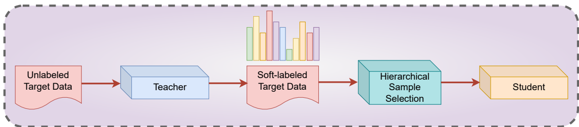
Figure 7. Teacher-student framework. The adversarially trained Teacher is used to annotate unlabeled target samples. Our hierarchical sample selection process picks a subset of samples to be used to train the Student model.
