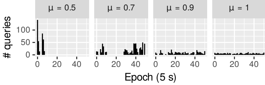
Figure 37. Number of queries submitted each 5-second epoch for example fractional Poisson query arrival processes with different “burstiness” parameter \mu . (Only first 50 epochs are shown for clarity.)
