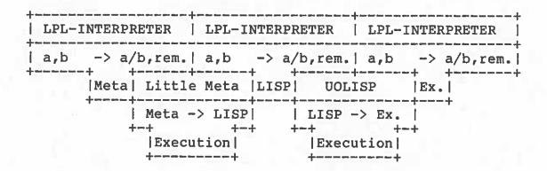
By turning on the UOLISP compiler we could actually cause the LPL-program to be converted from LISP into executable machine code. Our goal, however, is to implement an LPL-compiler which produces code capable of executing without the presence of the LISP interpreter. The LISP compiler generates code with many hooks into the LISP interpreter.
