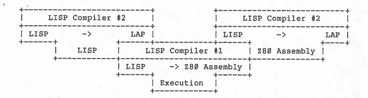
This composite diagram depicts the steps necessary to get LISP Compiler #2 into a form which can be executed. This is only possible with the assistance of LISP Compiler #1. Later on we will show how to "bootstrap" compilers using Little META.
