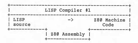
This diagram states that LISP Compiler #1 translates LISP source code into Z80 machine code. It also says that LISP Compiler #1 is implemented in Z80 Assembly language. When two or more translations of a program occur, a composite T diagram is used. Suppose that we have written LISP Compiler #2 in LISP which produces LISP Assembly Code (LAP). In order to get LISP Compiler #2 running we need LISP Compiler #1.
