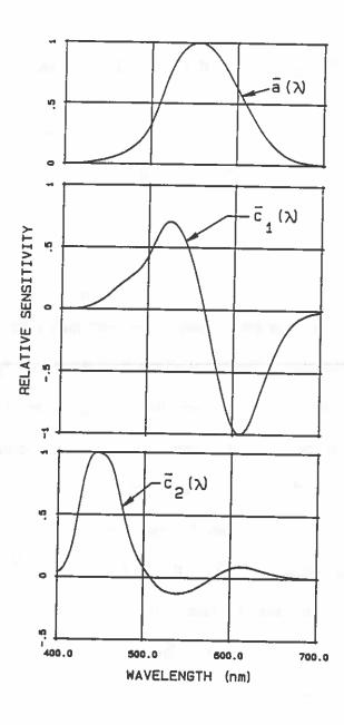
Figure 4: Spectral sensitivities for  $AC_1C_2$  space.
