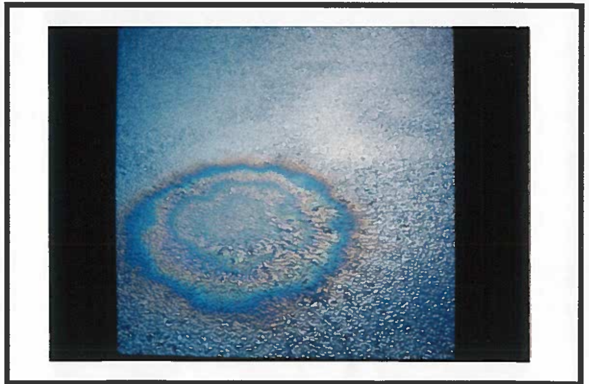
Figure 5: Simulation of the interference colors produced by an oil slick on wet asphalt pavement.
