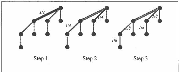
Figure 3: Phases in B(3) showing message volumes on active edges (highlighted)
