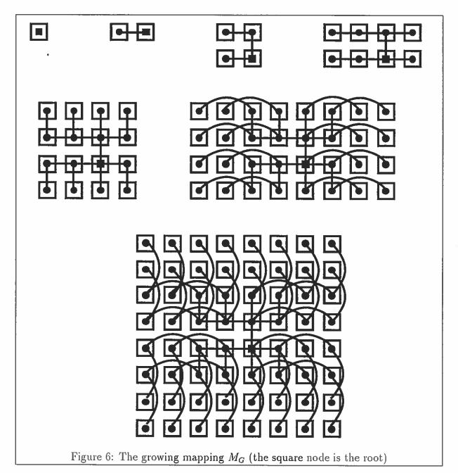
• If n = 2k, non-leaf nodes are mapped as a B(n-1) and leaves are 'grown' vertically from its parent with uniform dilation. Thus each node in the Northern (Southern) half of B(n-1) gets its leaf placed in the same column as itself at a distance  $2^{k-2}$
