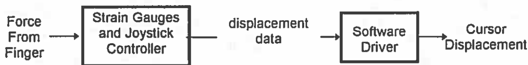
Figure 56. Block diagram of isometric joystick. (Modified reproduction of Figure 9).
