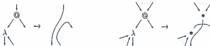
Figure 30. Beta-reduction principles for interaction nets and lambda-graphs
