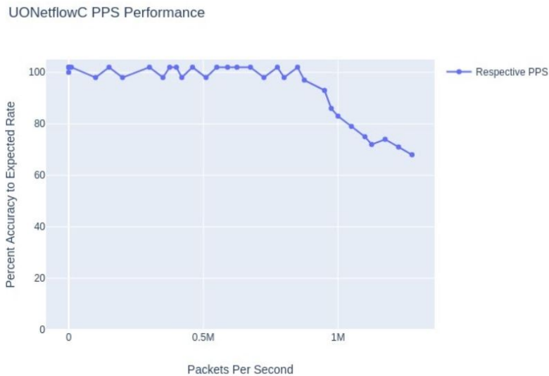
Figure 2. Netflow to Packet Synthesizer’s performance in PPS, run on Intel Xeon D-1548 2.0 GHz core, MLNX X-3 10 Gb/s NIC.
