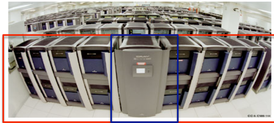
SGI Origin 2000 128 CPUs in NUMA configuration.
