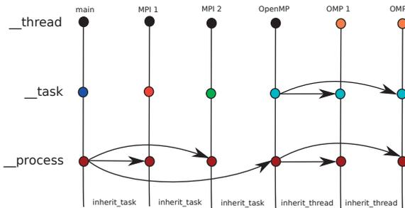
Figure 7: Two MPI Processes sharing the same OpenMP runtime.
