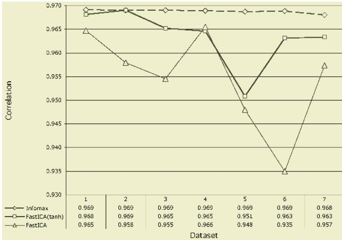
**Fig. 3.** Graph of correlations between original and ICA-filtered data across the seven datasets. Thin line, FastICA with cubic contrast function. Thick line, FastICA with tanh contrast function. Dotted line, Infomax.
