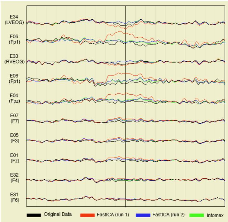
**Fig. 6.** EEG waveforms, averaged to the peak of the blink activity. Note residual blinks in run 1 for FastICA, where more than one source was strongly correlated with the blink template, and the source activations revealed misallocation of variance (cf. Fig 5).
