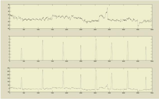
**Fig. 2.** Construction of "synthetic" data. Top panel, original data (~10 sec). Center panel, simulated blinks (Dataset #7). Bottom panel, original data plus simulated blinks.
